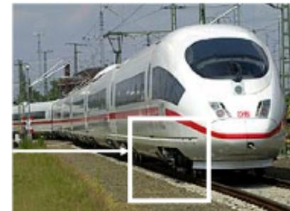
A piezoelectric sensor detects the vibrations of the wheel, leading to an assessment of its wear status
