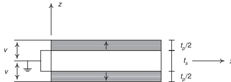
Electrical connections for a piezoelectric extender actuation. A voltage is applied to the piezoelectric layers aligned with the poling direction of both piezoelectric layers
