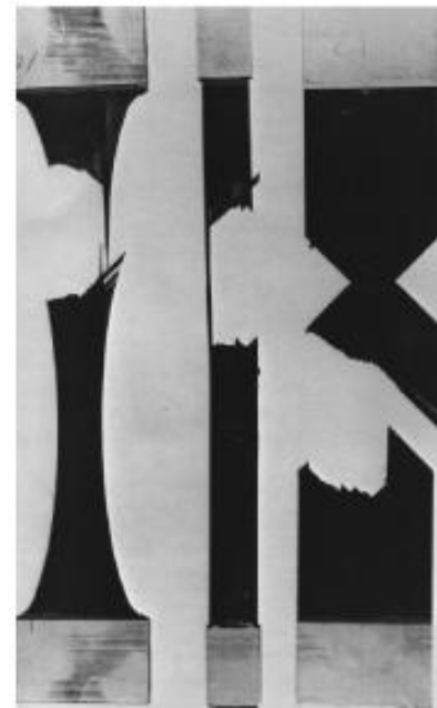
Figure 2 Coupons with varying gauge profiles tested: (a) statically, (b) fatigue.
